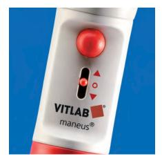
The pipetting knob allows sensitive intake and delivery of fluids. For blow-out pipettes press the discharge bellows for emptying (blow-out) which is coloured in red like all functional elements.
